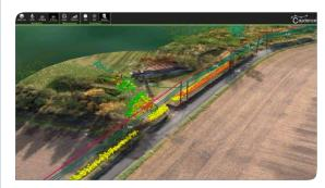
The aerial laser scanning system is much faster than foot-patrolled line inspections and allows inaccessible areas to be monitored more effectively.
